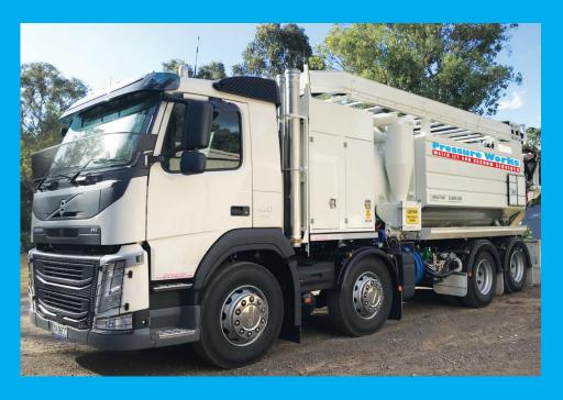
lower overall height the overhead cassette has 20 metres x 6" vacuum hose and the long reach 'simultaneous' boom raises to 5.2m and 180° rotation.
